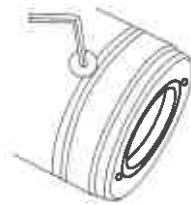
Tighten the cover anti rotation screws
