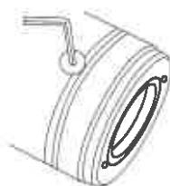
Tighten the cover anti rotation screws
